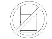
The VESDA-E detector can be mounted in an upright or inverted position. Do not mount the detector with a sideways orientation.
