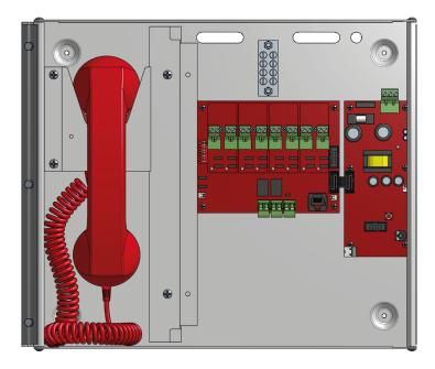
Prior to mounting the Crisis EVC Standalone Master Station, it should be decided if the field wiring is to be run on the surface or concealed. There are 14 knockouts on the top and 2 slotted entries with a dedicated mains supply entry at the rear. If a knockout is removed by mistake, fill the hole with a good quality cable gland.
