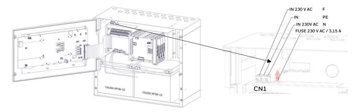
The connection to the 230 V AC power supply mains must be performed through three-conductor cable (phase- neutral- earth).
