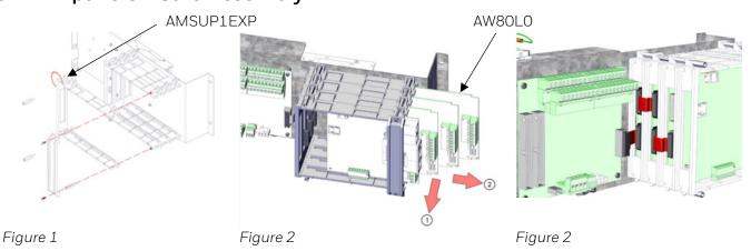
Kit AMSUP1EXP to install additional loop cards to expand the panel up to 8 loops. Once fixed the additional kits as shown in figure 1, LIB Cards could be insert into the slot as shorn in Figure 2 and then connected with the flat cable from LIB #1 as shown in Figure 3.
