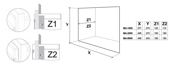
**Step 1:** create a recess in a wall into which the MAX panel is to be semi flush mounted. The Recess Depth Z1/Z2 must be such that there is clearance to allow door to work.
