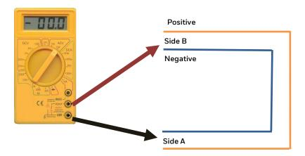
The direct current resistance of the negative wire of the loop SHALL NOT exceed 20 Ohm.
