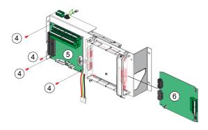
4. Unscrew the 4 x screws @ from the board © and remove all existing boards © installed into the panel.
