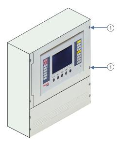
3. Remove the 2 screws ① and open the panel door.
