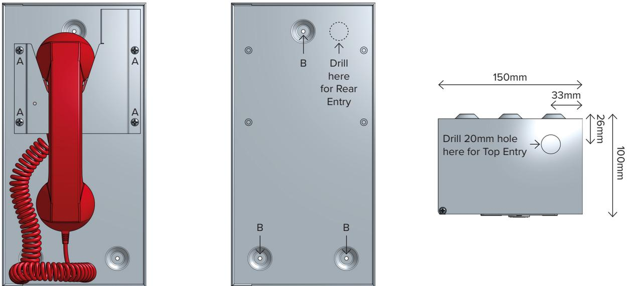
Figure 1: Fixings and Cable Entries
